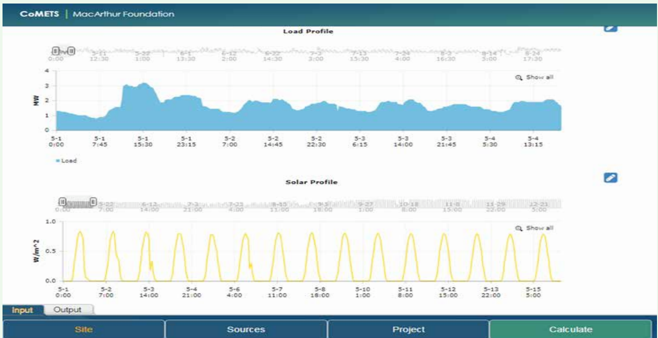
Figure 23: Load and Irradiance data dashboard
