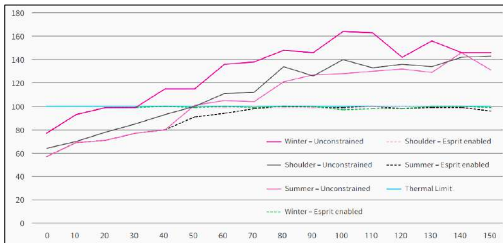
Figure 2.18: Unconstrained and Esprit enabled network impacts with increasing EV penetration levels, (x-axis: EV penetration (in %), y-axis: thermal capacity utilized (in %))(My Electric Avenue - Project Close-Down Report, 2016)
